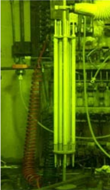
Seven irradiated Cm targets in hot cell
